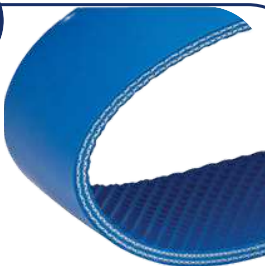
PVC 3.3 mm Diamond 2 Ply. ( Glossy ) Min. Pulley Dia. 95 mm.
