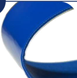
PVC 2 mm Blue 2 Ply. ( Glossy ) Min. Pulley Dia. 30 mm.
