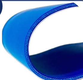
PVC 3 mm 2 Smooth Blue 2 Ply. ( Matt Surface ) Min. Pulley Dia. 120 mm.
